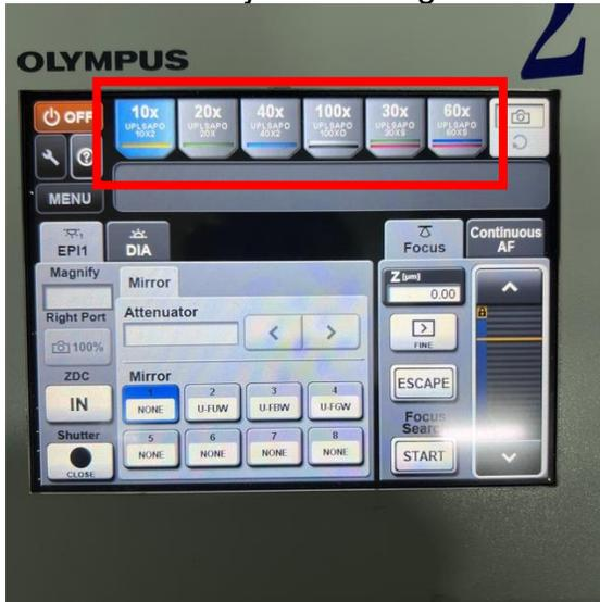
**Make sure the correct immersion medium is used for the objective you selected (Air/Oil/Silicone oil).**
