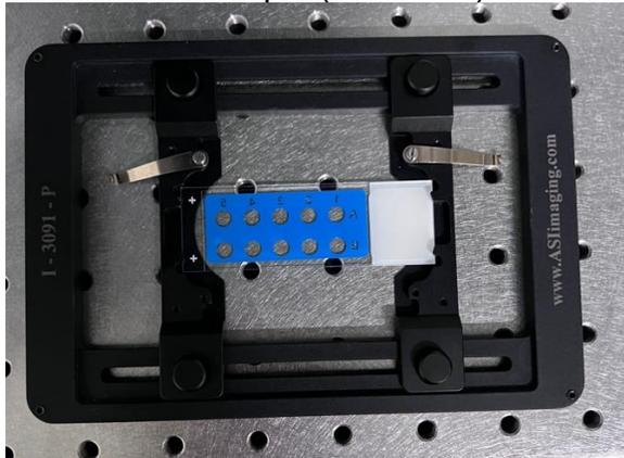
4. Place the sample-loaded stage holder on the ASI microscope stage.
