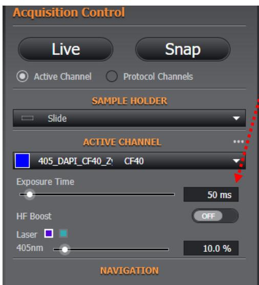
2. After the sample is in focus in live view, adjust camera exposure time and laser power for optimal imaging quality with this channel.
