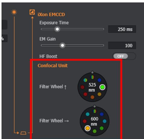
For 488/561 simultaneous acquisition, the positions of the two filter wheels should be 525nm for cam2 (Filter Wheel ↑) and 600nm for cam1 (Filter Wheel →).
